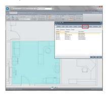
Data relating to Graphical Non-Clickable Assets assigned to a space on a drawing can be retrieved & reported while working in the EvolveFM Drawing Viewer and this technique adds the ability to see a graphical representation of the asset on the drawing. they cannot see the physical representation of the asset on a drawing. These types of assets usually consist of the items you need to track for Human Resource purposes, inventory purposes, and large equipment items.
